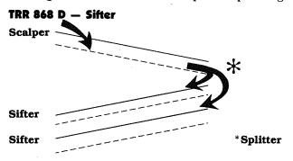
The commodity falls through the top scalping screen while large foreign material is discharged over the screen. The good product enters the splitter where the flow is evenly divided . . . half to each sifting screen. The good product travels over these screens as splits and undersized foreign material sifts through.
