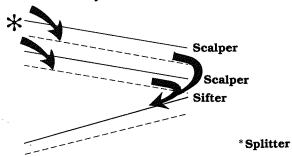
The commodity is split-fed, half to each of the two top scalping screens. Large, bulky trash is scalped off as the good product falls through. Since each screen handles only one half the total volume, closer perforations can be used. The third screen holds up the good product while light trash, weed seeds and splits drop through.
